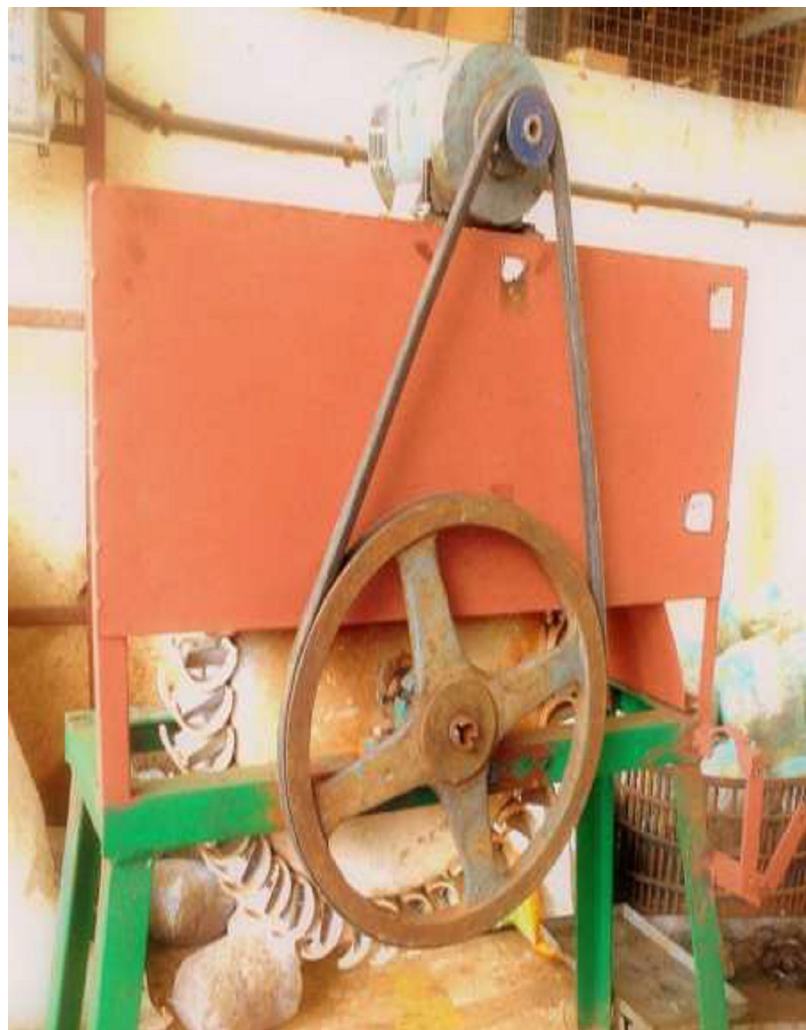
Plate.3 Small pico-hydro power generation unit
